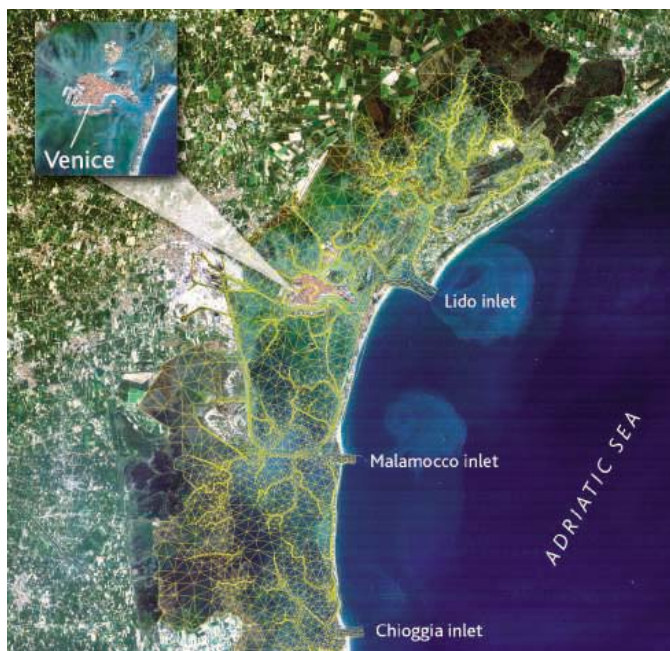
Complex interactions. A computer model, overlaid on a satellite image, divides the Venice Lagoon into thousands of interacting triangles to enable study of its processes, such as water flow and sediment transport.
